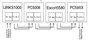
For example, if you are installing a PC1555MX with a LINKS1000 and a PC5928 Intercom module, connect the incoming line to the LINKS1000, then from the LINKS1000 to the PC1555MX, then from the PC1555MX to the PC5928 Intercom and then from the PC5928 to the house telephones.
